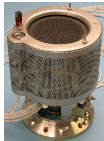
Figure 6.10: The Qinetiq T5 ion thruster [5]
