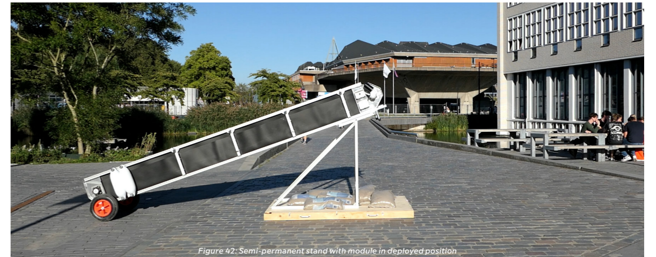
Figure 42: Semi-permanent stand with module in deployed position
