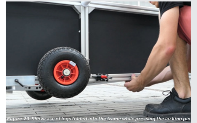
Figure 29: Showcase of legs folded into the frame while pressing the locking pin
