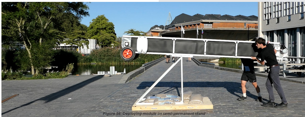
Figure 56: Deploying module on semi-permanent stand
