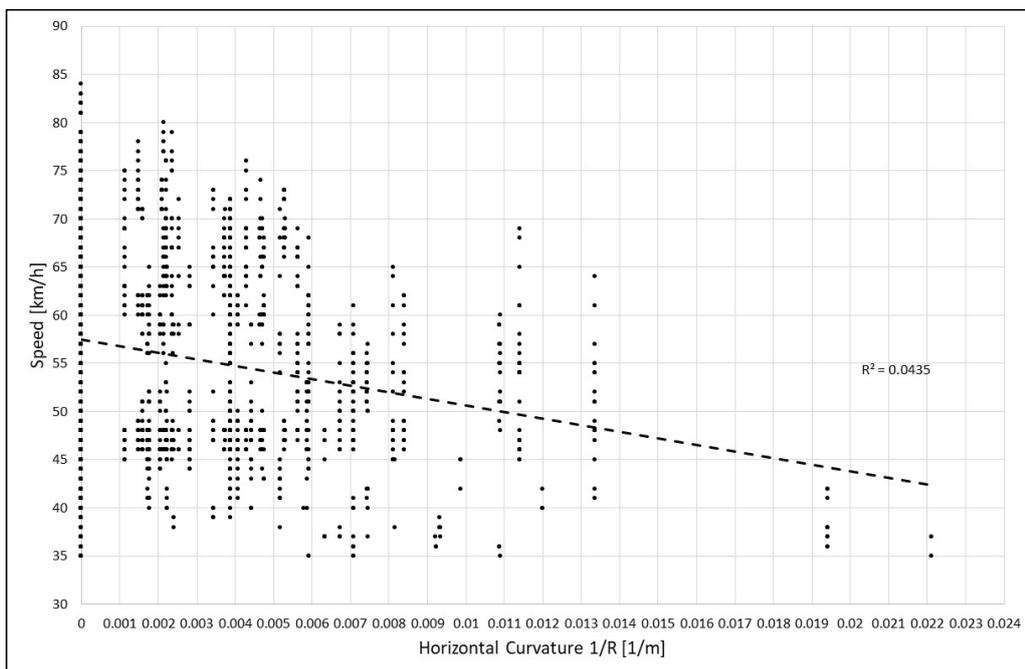
211 **Fig. 3 Variability of speed vs. horizontal curvature**
