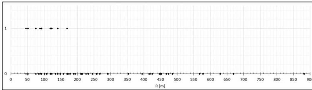
Fig. 4 LSS fault (value=1) vs. horizontal curvature
