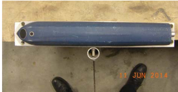
Figure 3.25 The acoustic profiler used by Hemmerle et al. (2014) and Cedillo et al. (2016). Source: Hemmerle et al. (2014).
