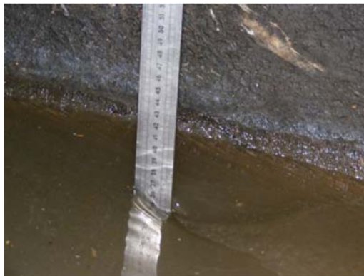
Figure 3.8 Not so easy to read a ruler! Water level of 36 cm upstream, 35 cm downstream. Source: Université Gustave Eiffel.
