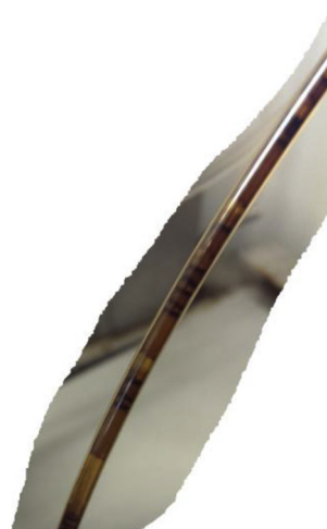
Fig. 12. Fluids at the outlet of the core; appearing more like an emulsion than a foam.
