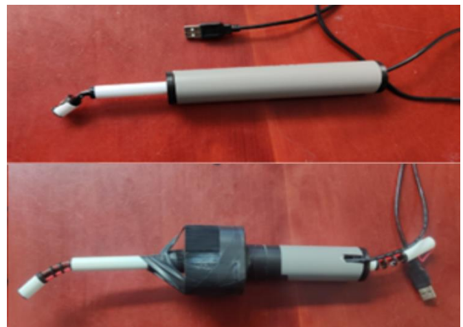
Figure 9: Intermediate prototypes of FlexEye laparoscope (top) and the Flip laparoscope (bottom)
