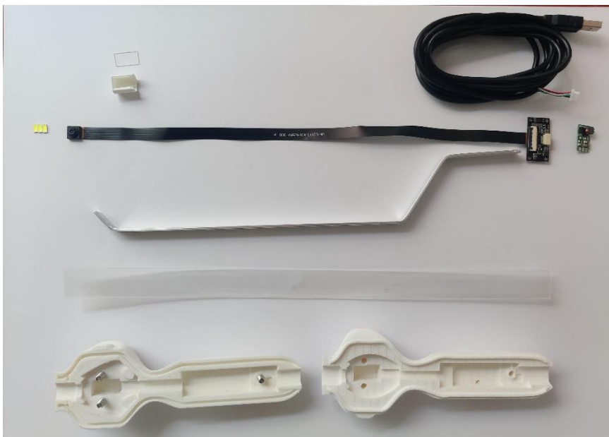
Figure E: Components produced for the updated gasless laparoscope.
