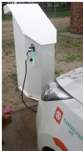
Fig. 5 V2G-DCAC unit connected to the FCEV.
