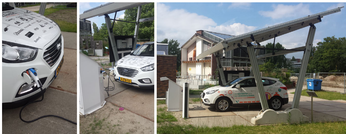
Fig. 1 Experimental Fuel Cell Electric Vehicle-to-Grid (FCEV2G) set-up at The Green Village, Delft University of Technology, Delft, The Netherlands.
