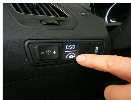
Fig. 4 New dashboard V2G activation button also initiates Cold Shut Down.
