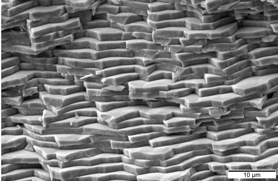
Figure 1.6: Scanning electron micrograph of blue mussel ( Mytilus edulis ) nacre (cross-section).
