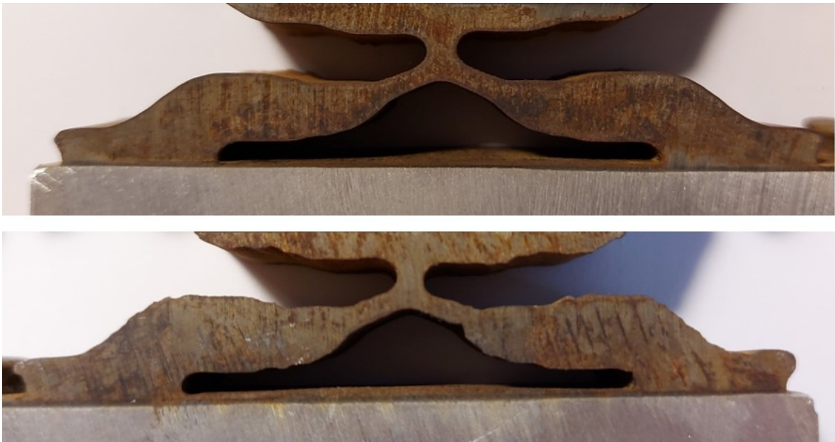
Figure 5-3: Visualization of the difference between the surface finish at the front (top) and rear (bottom) of the manufactured sample. The front of the sample is the side from which the waterjet perforated the sample.
