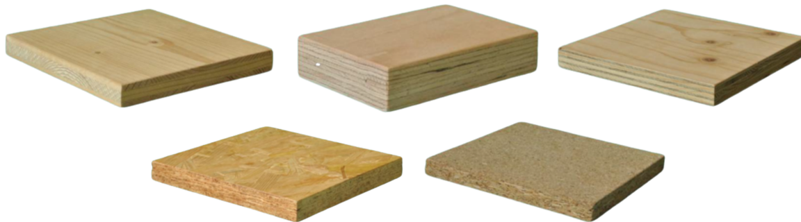
Figure 2.3: Examples of wood-based panels (Top: solid wood panel, LVL and plywood. Bottom: OSB and particleboard) (Joachim Blaß and Sandhaas, 2017, p. 121-128)
