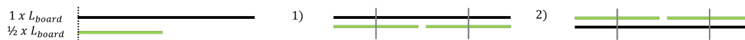
Figure D.1: Different segments for a two layered system with two fasteners per plate
