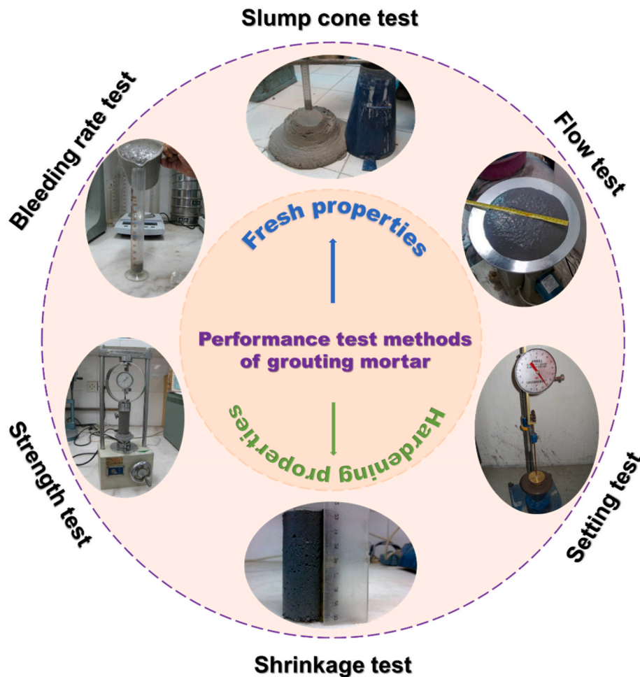
Fig. 5. Performance test methods of grouting mortar.
