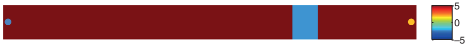
Fig. 1—Permeability field of a 1D homogeneous reservoir model with a low-permeability barrier. Permeability values are expressed as the natural logarithm of permeability in md. The blue and orange dots indicate the injector and the producer, respectively.
