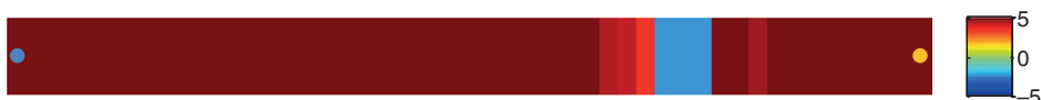
Fig. 3—Updated permeability field of the 1D reservoir model for Experiment No. 1. Permeability values are expressed as the natural logarithm of permeability in md.
