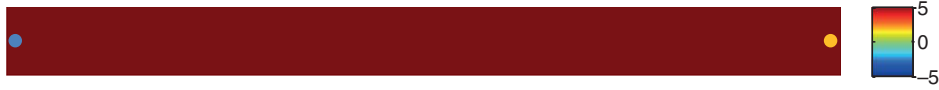
Fig. 2—Permeability field of the starting model. Permeability values are expressed as the natural logarithm of permeability in md. The blue and orange dots indicate the injector and the producer, respectively.
