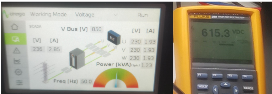
Figure 5.6: AC source and DC output voltage measurements
