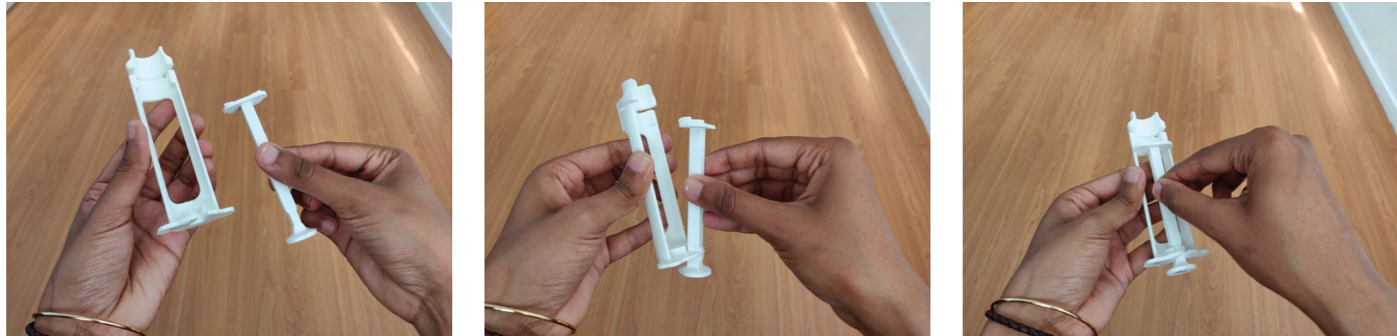
Fig. From left to right a) The Chloe SED before assembly b) and c) Inserting the plunger
