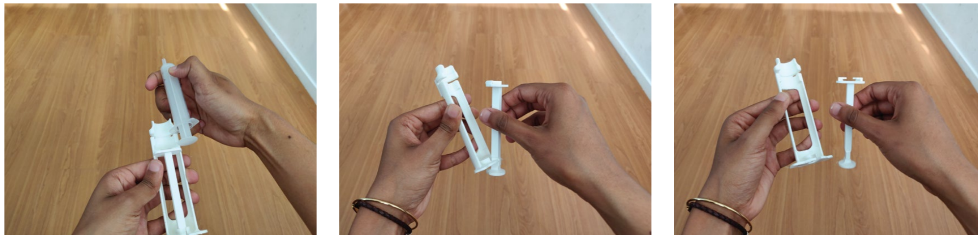
Fig. From left to right a) Disassembling the Syringe from SED b) Disassembling the plunger and body of the SED
