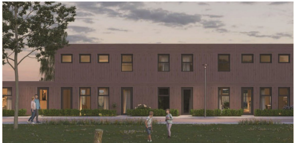
Figure 8. The modules are available in numerous configurations with different facades. Source: Dura Vermeer.
