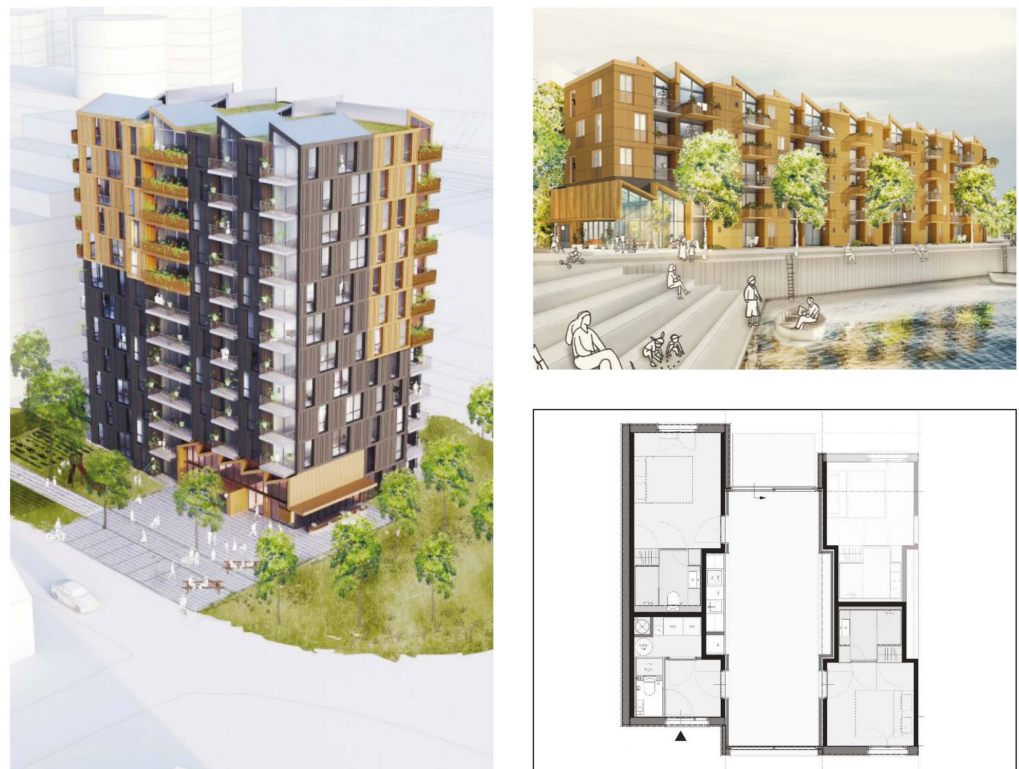
Figure 6. Left, MOOS as multi-storey apartment building up to 70 m height. Right above, a multi-storey building without a lift. Right below, three different modules of MOOS. Source: In the Middle of Our Street.
