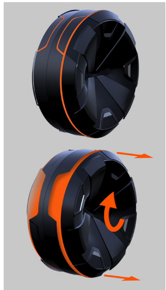
Figure 11.1 // Explanation sketch of the wheel concept
