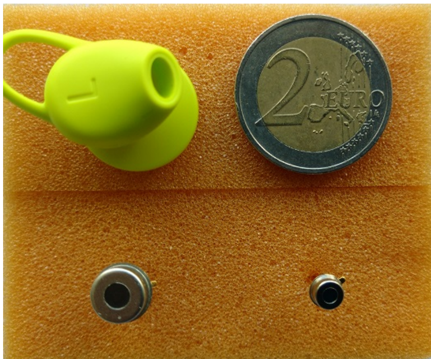
Figure 3.3: Size comparison of an earpiece, a 2 Euro coin, a TO5 sensor and a TO46 sensor
