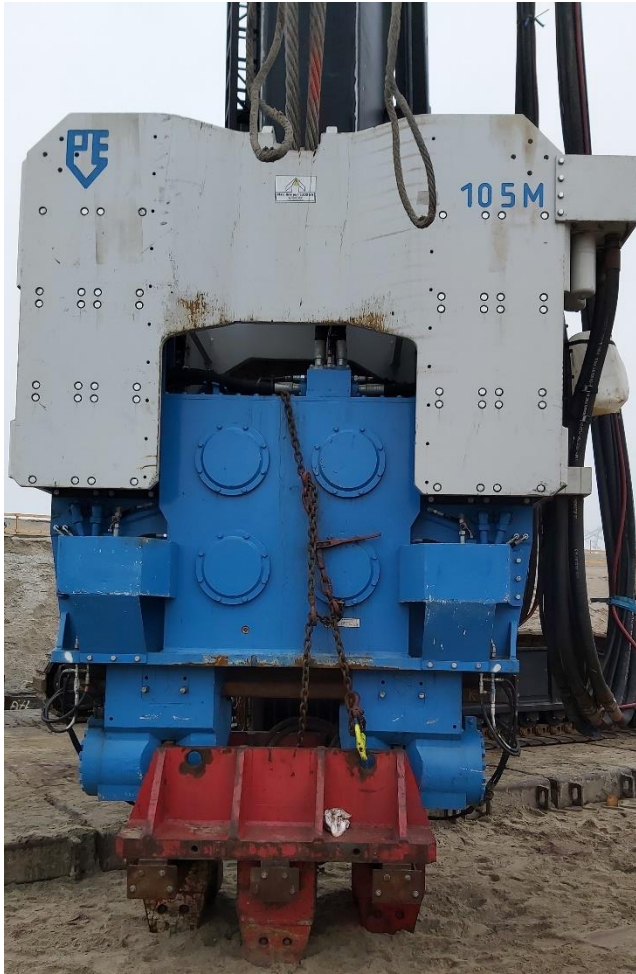
Figure A 1: Vibratory hammer (photo personally taken).
