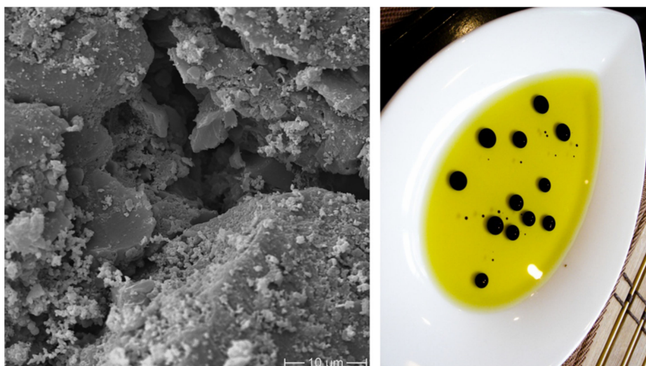
Figure 2. Chemical Purification; examples of adsorption and phase separation: (Left) Active charcoal. Scanning electron microscopy micrograph of activated charcoal showing the large available surface area resulting in high adsorbability. (Right) Phase separation of oil and vinegar. Hydrophobic oil and hydrophilic vinegar separate into two different phases, which can be used to filter one out of the other (images adapted from Wikipedia common. (Left) Wikimedia Commons contributors, “File:Activated Charcoal.jpg,” Wikimedia Commons, the free media repository, https://commons.wikimedia.org/w/index.php?title=File:Activated_Charcoal.jpg&oldid=417429816 ; (Right) Wikimedia Commons contributors, “File:Olive oil with Balsamic Vinegar.jpg,” Wikimedia Commons, the free media repository, https://commons.wikimedia.org/w/index.php?title=File:Olive_oil_with_Balsamic_Vinegar.jpg&oldid=331512136 (accessed 17 June 2020).
