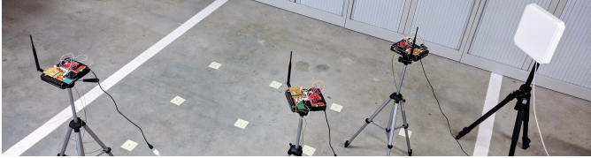
Fig. 9. Photograph of the setup to evaluate phase cancellation countermeasures in T2T networks, discussed in Section VII-C: Three backscatter T2T tags on tripods, next to white panel antenna; grid coordinates marked with yellow squares on the floor.
