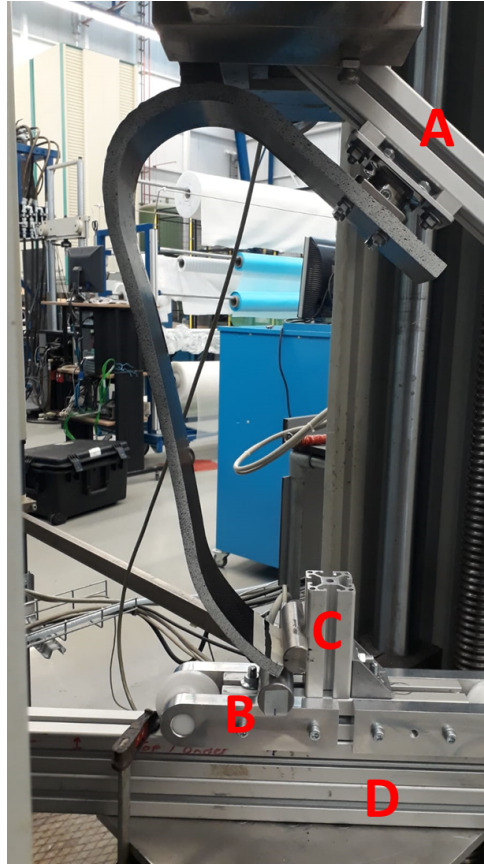
Figure 2.14: Static compression test set-up. A is the attachment to the prosthesis that allows the rotation of the prosthesis ensuring that the point of attachment to the test bench and the contact point are vertically aligned. B is the slider that allows the horizontal displacement ensuring that the contact point does not change during the test. C is the vertical aluminum profile that ensures that there is no relative movement between the prosthesis and the slider. And D is the aluminum profile over which the slider translates.
