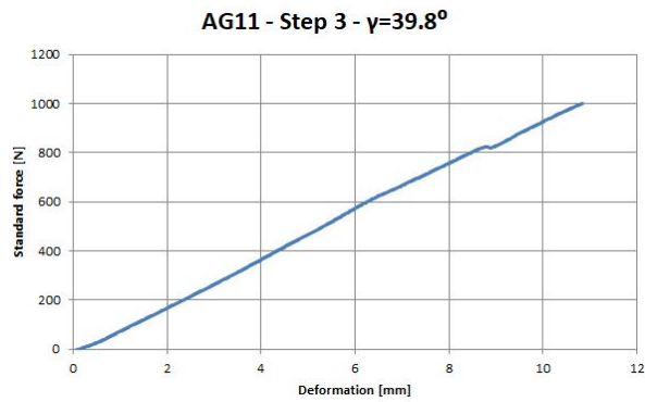
Figure K.16: AG11 - Step 3 - \gamma = 39.8\text{deg} . Test bench vertical stiffness plot.
