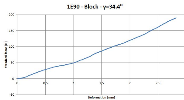
Figure K.46: 1E90 - Block - \gamma = 34.4deg . Test bench vertical stiffness plot.
