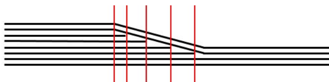
Figure F.2: Illustration of the partitions created in the Abaqus shell to simulate dropping plies. Creating 5 partitions divides the laminate in 6 different sections, what allows to choose a different lamination for each of the sections in Abaqus. The first section starting from the left is assigned 8 plies; the second section, 7 plies; the third section, 6 plies; and so on. This is how the ply drops were mimicked in Abaqus.
