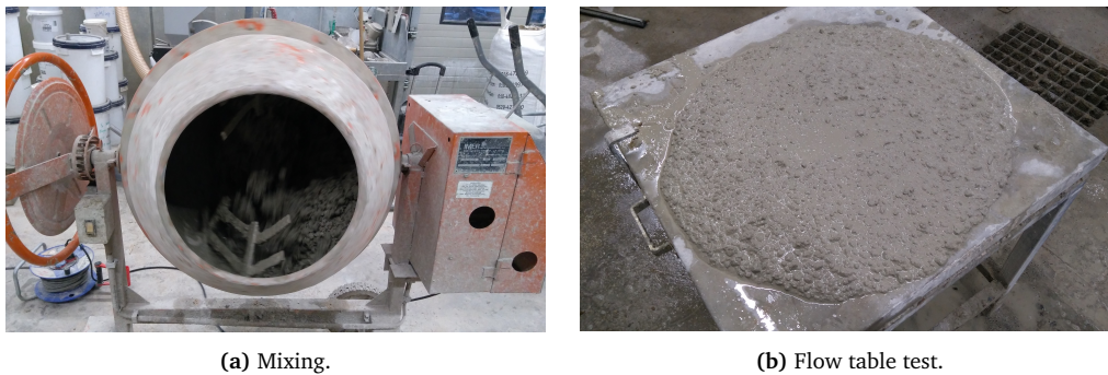
Figure 4.1: Fresh concrete handling.
