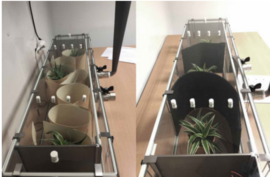
FIG. 3.3 Selected materials + Spider plant inside of the CLIMPAQ 50L.
