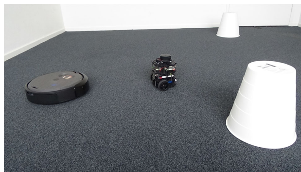
Fig. 12 A view of the scenario of the experiments, with the robots (the TurtleBot used as the SaR robot is in the middle and the iCreate3 robot used as the victim is at the side) and the obstacles (white buckets)
