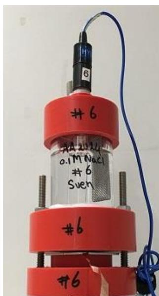
Figure 3. 5: Custom three-electrode electrochemical cell.
