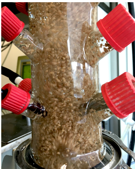
Figure 6.10: Section of a bubble column reactor, containing enriched granular biomass. Several different applications of granular biomass are under investigation. Possibly the simplest system to start exploring omics tools with is anaerobic VFA production from glucose [45]. Photo from personal archive.
