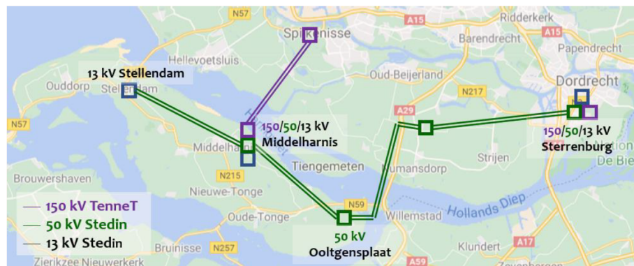
Figure 3.1: 50 kV grid lay-out with the 50/13 kV transformers of Stedin and 50/150 kV transformers of TenneT on Goeree-Overflakkee [33].
