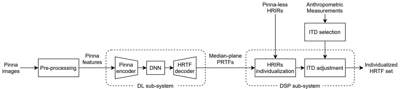
Fig. 1. HRTF individualization system. Figure reproduced from [13].
