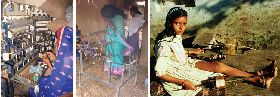
Figure 2-11 and 2-12: The Tasar silk reeling and re-reeling machines as introduced by PRADAN Figure 2-13: Thigh reeling, a traditional method of Tasar yarn reeling (picture by PRADAN)
