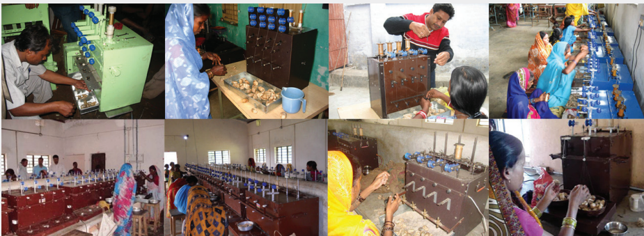
Figure 2-14 (a-h): Several prototypes of the Anna Tasar Reeling Machine (pictures c-h by MASUTA)
