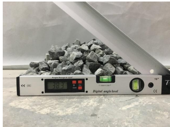
Fig. 4 (a) Ballast particle size distribution, (b) Repose angle of ballast.
