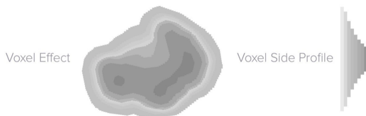
Figure 17. Effect of voxels on curved lines [31]
