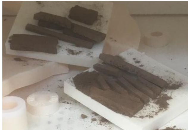
Figure 54. DLP sintered samples
