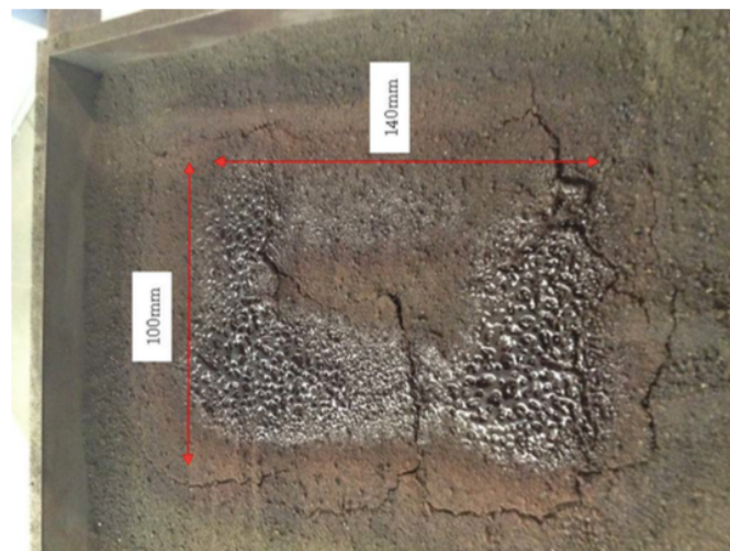
Figure 27. 2D unhomogeneously sintered part of as-received JSC-1A regolith simulant [9]
