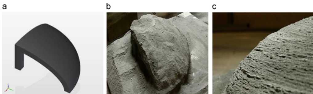
Figure 30. (a) 3D drawing of the convex artifact, (b) unpolished printed piece built using the DNA-1 simulant (395 mm x 395 mm x 195 mm) and (c) particular of the artifact surface after dust removal [7]
