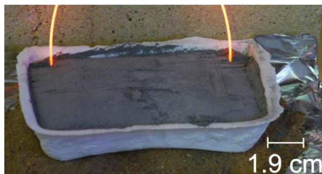
Figure 9. Heating procedure of mixture of regolith and aluminum [21]
