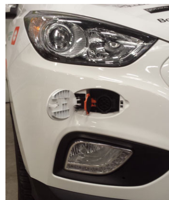
Fig. 3 V2G Type 1 Socket integrated in the front bumper.
