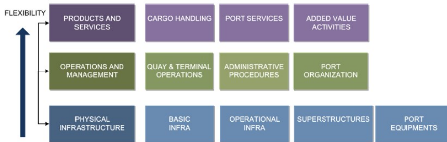
Figure 1.1: Three-layer inframodel of a port; by Herder et al. (2008) and adapted by Dr. Taneja [42]
