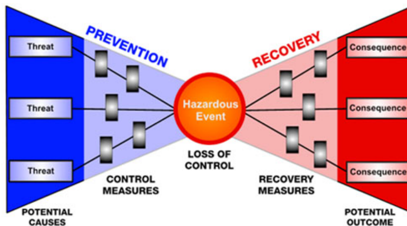
Figure 4.3: Example for the Bow-Tie Method.
