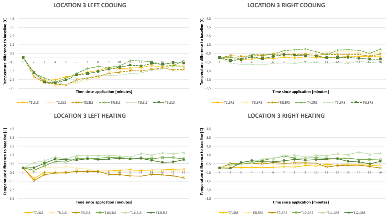
Figure 17: Cooling versus Heating Location 3. The tests with the cooling agent are represented with a dashed line and those for the heating agent with a solid line. The green lines represent tests where the agent was applied to the palmar side and the yellow lines the tests where it was applied to the dorsal side. The abnormal line T9L1LS belongs to test nine which is unreliable as described earlier.
