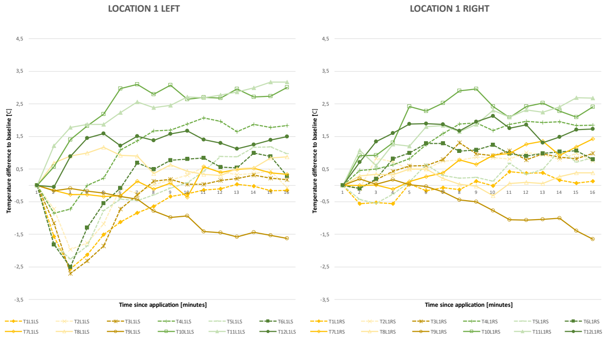
Figure 7: Location 1 Left - Right Difference. Tests 1 to 6 were done with the cooling agent, test 7 to 12 with the heating agent. Each line is an averaged test run with the following naming convention: TxLyLz where x is the number of the test, 1-12, y is the location, 1-4, and z is the side, LS left or RS Right. The tests with the cooling agent are represented with a dashed line and those for the heating agent with a solid line. The green lines represent tests where the agent was applied to the palmar side and the yellow lines the tests where it was applied to the palmar side. The abnormal line T9L1LS belongs to test nine which is unreliable as described earlier.
