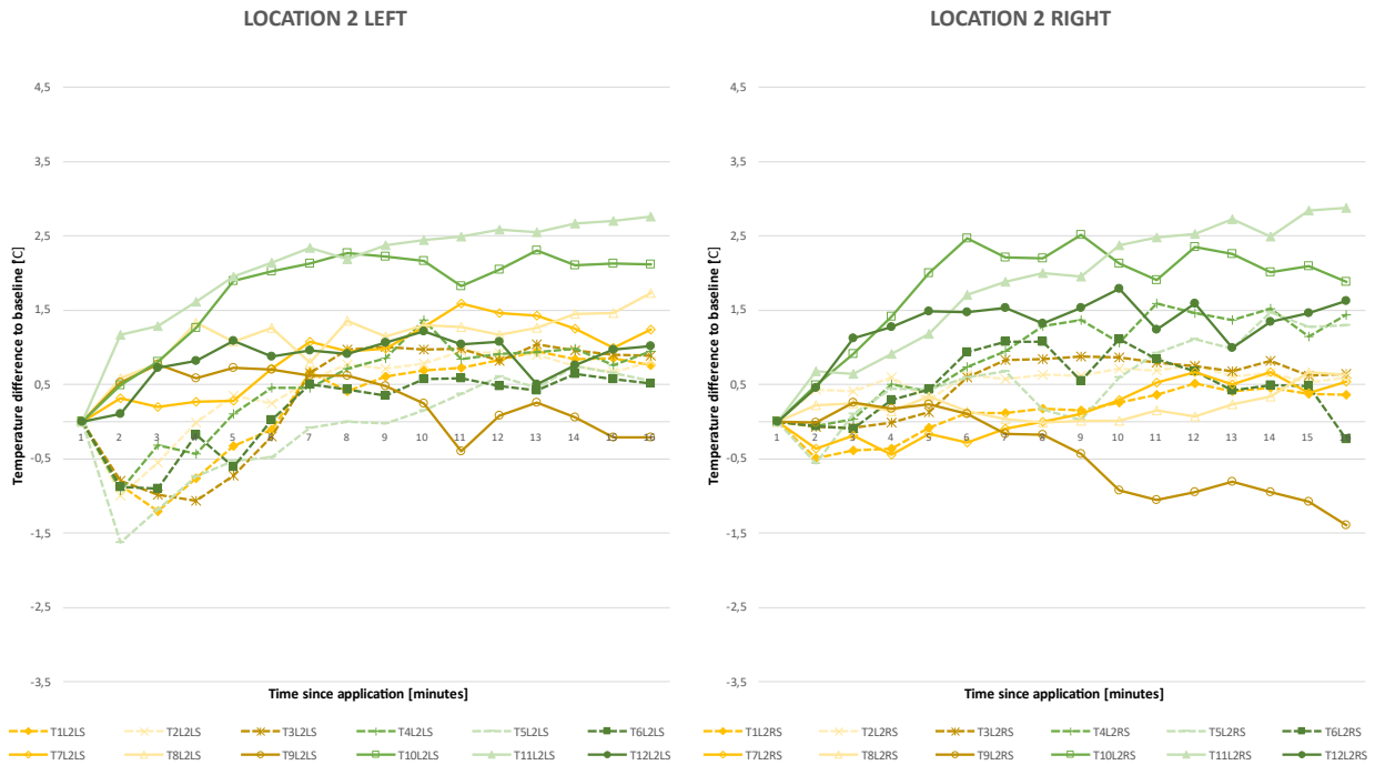
Figure 8: Location 2 Left - Right Difference. Tests 1 to 6 were done with the cooling agent, test 7 to 12 with the heating agent. Each line is an averaged test run with the following naming convention: TxLyZ where x is the number of the test, 1-12, y is the location, 1-4, and z is the side, LS left or RS Right. The tests with the cooling agent are represented with a dashed line and those for the heating agent with a solid line. The green lines represent tests where the agent was applied to the palmar side and the yellow lines the tests where it was applied to the palmar side. The abnormal line T9L1LS belongs to test nine which is unreliable as described earlier.
