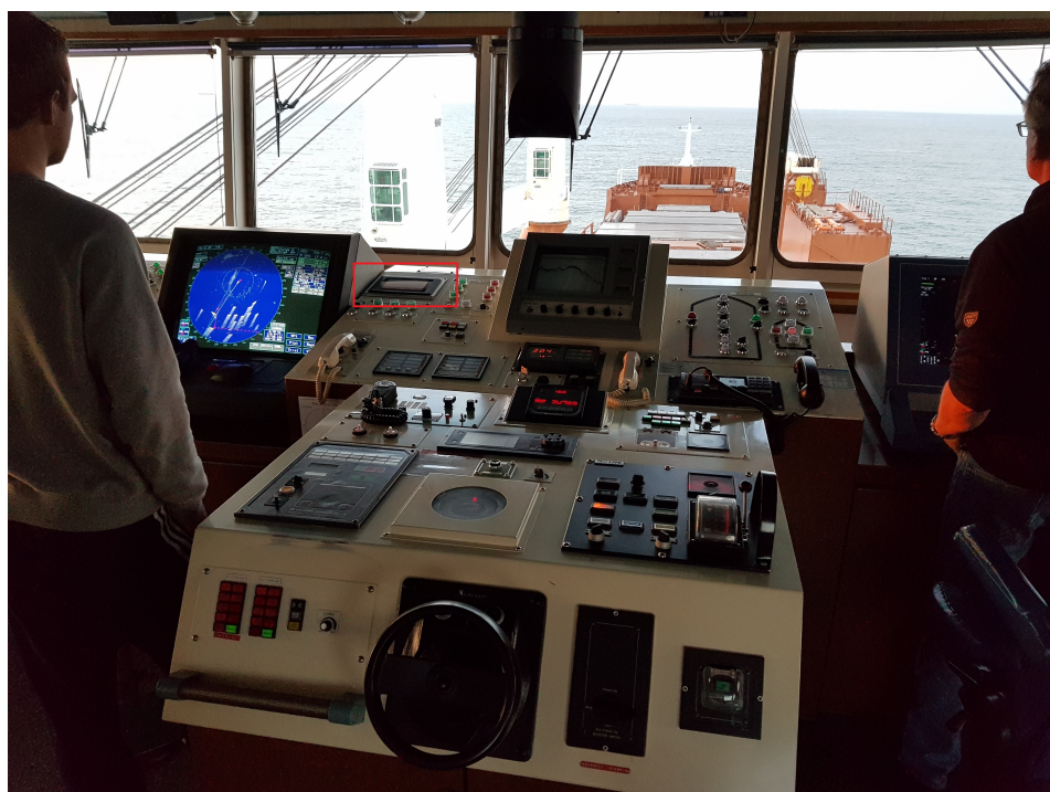
Figure 4.5: Bridge of the MV Schippersgracht with Performance Indicating System boxed in red
