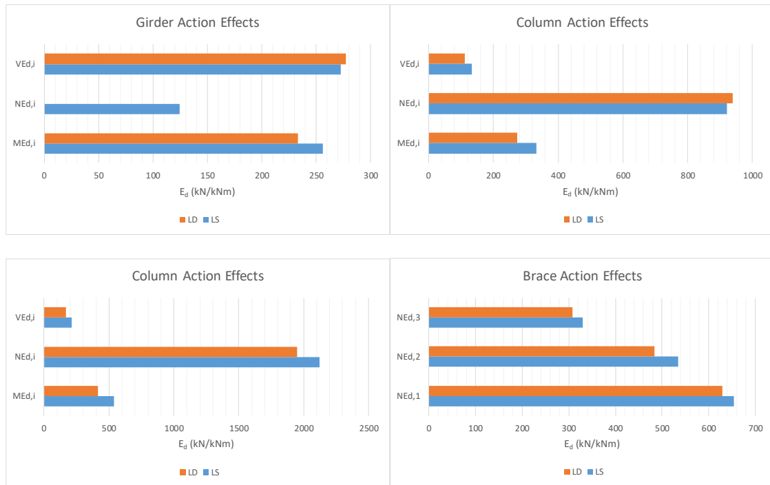
Figure 5.2 Comparison of critical element forces from linear static (LS) and linear dynamic (LD) procedures for a) MRF girders, b) internal MRF columns, c) external MRF columns and d) axial forces in braces
