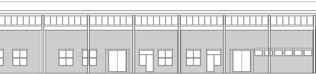
Innovation Factory - New South elevation 1:200
