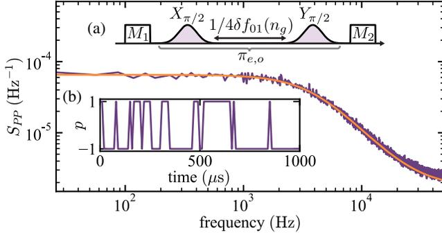
FIG. 3. Detecting fast charge-parity switches in an offset-charge-sensitive transmon qubit. (a) Charge-parity-mapping pulse sequence, which results in an effective charge-parity-conditioned  $\pi$  pulse,  $\pi_{e,o}$ . Inset (b): A 1-ms snapshot of a  $\sim 600$ -ms-long charge-parity jump trace. Main: Power spectrum of charge-parity fluctuations, with a Lorentzian fit (orange curve) corresponding to  $T_p = 77 \pm 1 \mu\text{s}$ .
