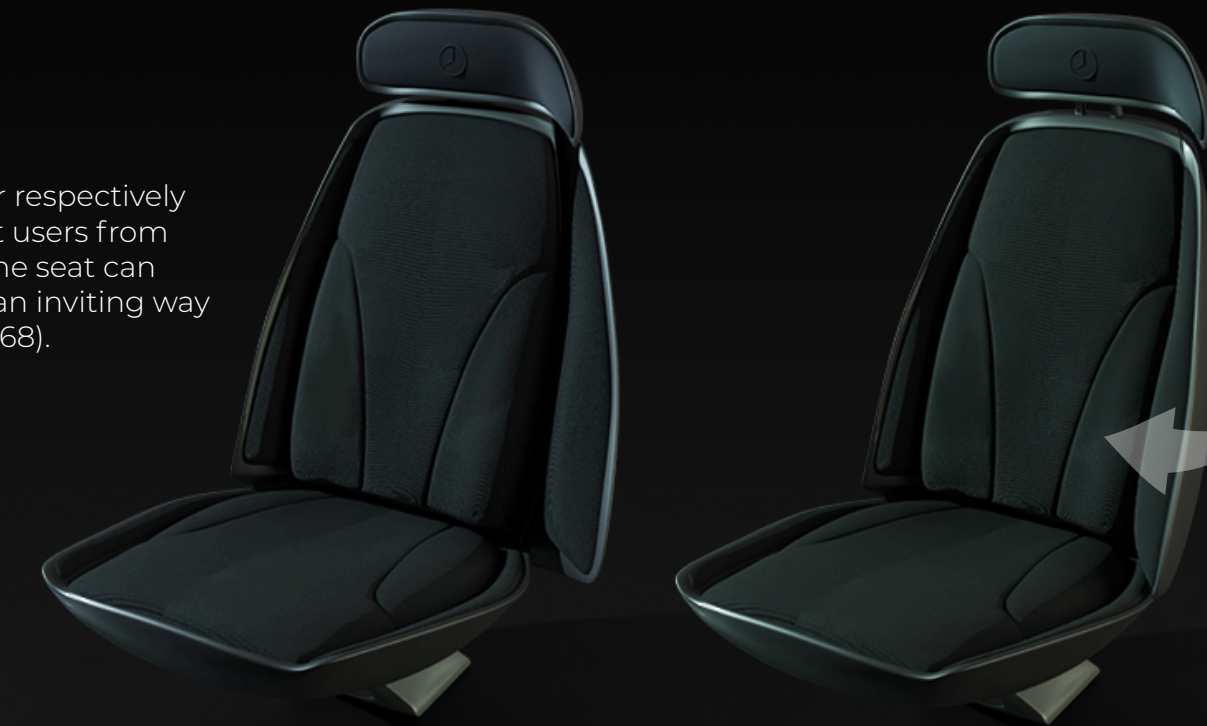
Figure 68 | Opening Chair Flap for Getting in and out of the Car
