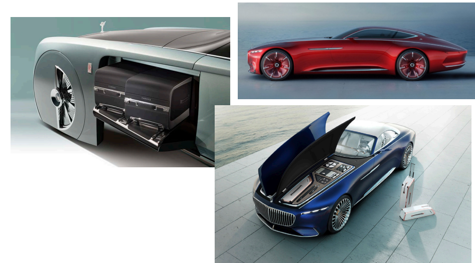
Figure 26 | Rolls-Royce Vision (left) & Maybach Vision 6 (right): Obtaining Prestige Length by Repurposing Bonnet as Stowage Area
