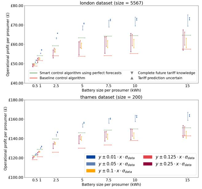
Figure 5: High-level comparison between operational profits of the baseline algorithm and smart algorithm for the average prosumer using various battery sizes and lookahead amounts with uncertain forecasts based on linear margins.
