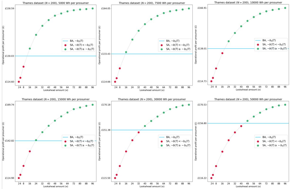
Figure 13: Overview of operational profits per prosumer for the baseline- and smart control algorithm using various sizes for the lookahead window ( $\kappa$ ) and various sizes for the battery per prosumer ( $\omega/N$ ) on original historical data of Thames (part 2).
