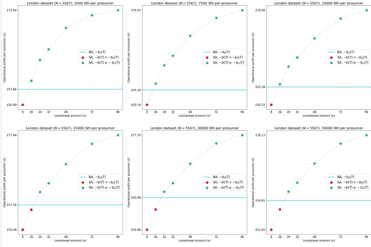
Figure 11: Overview of operational profits per prosumer for the baseline- and smart control algorithm using various sizes for the lookahead window ( $\kappa$ ) and various sizes for the battery per prosumer ( $\omega/N$ ) on original historical data of London (part 2).
