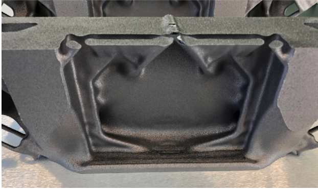
Fig. 19. The first print attempt, showing the locally overheated and deformed parts, causing recoater damage.
