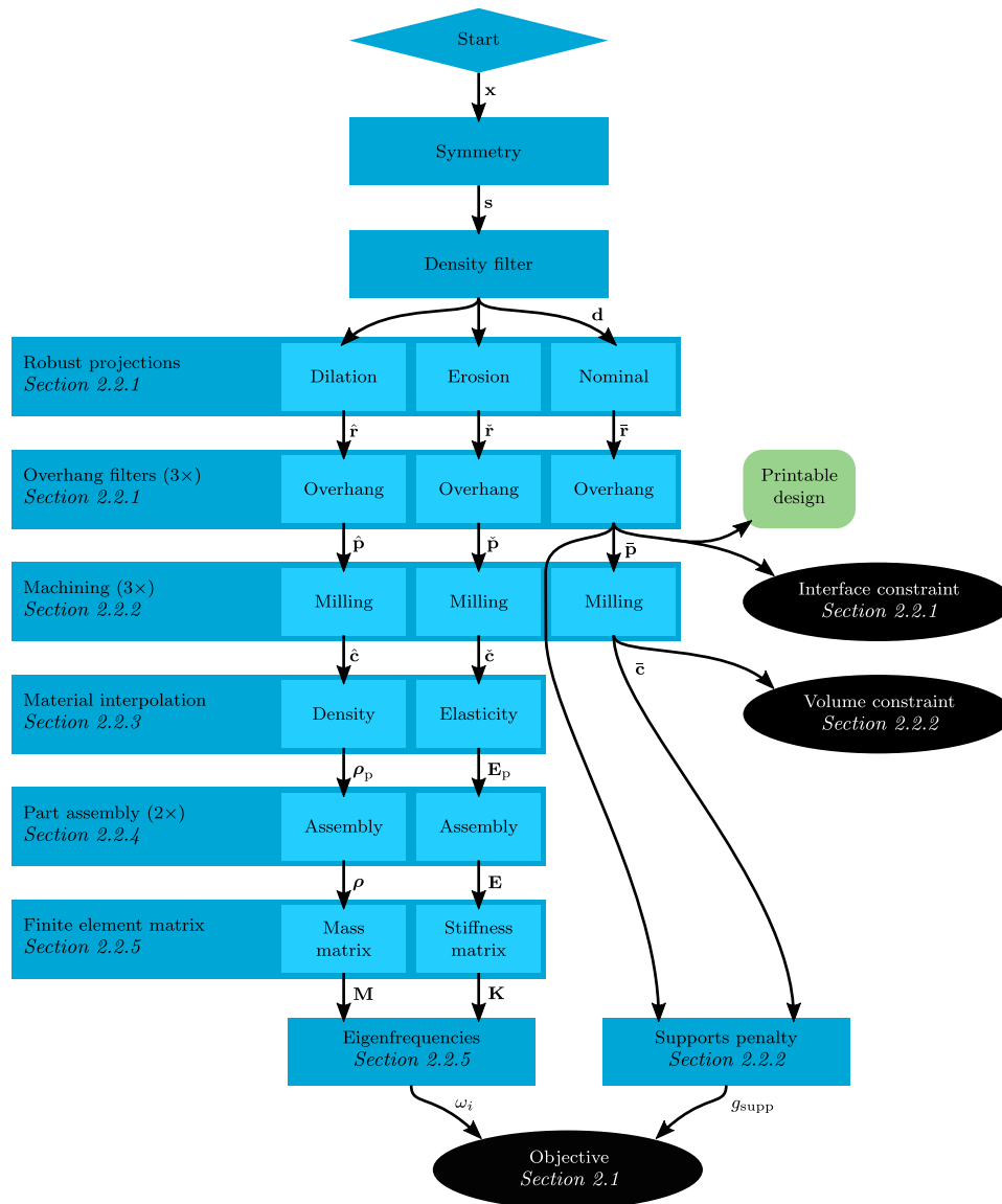
Fig. 2. Graphical overview of the optimization formulation as a flowchart (Eq. (1)). The design variables x are passed through a sequence of filters and mathematical operations (the blue blocks) in order to obtain the objective and constraint values (in black) corresponding to a manufacturable design. The entire sequence of operations is executed in each design iteration, where the optimizer repeatedly determines the new design x . The design used for actual printing is indicated in green. The individual operations are explained in detail in corresponding sections. (For interpretation of the references to color in this figure legend, the reader is referred to the web version of this article.)
