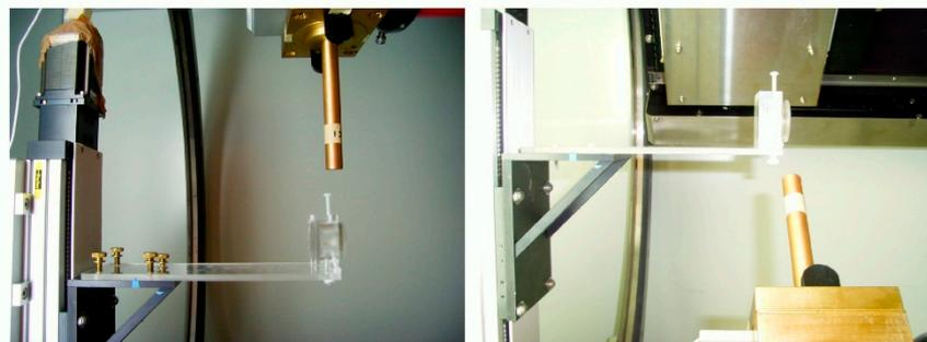
**Figure 9. Upper:** the PMMA RFG cell holder with a 20 mm thick RFG gel in a 50 mm diameter quartz cell for measurements in a “small animal” microbeam X-ray irradiation facility at the Antonie van Leeuwenhoek Ziekenhuis (Nederlands Cancer Institute) Amsterdam. **Lower:** a 6 mm gel positioned under the beam collimator, which could be rotated over 360 degrees in the X/Y plane.
