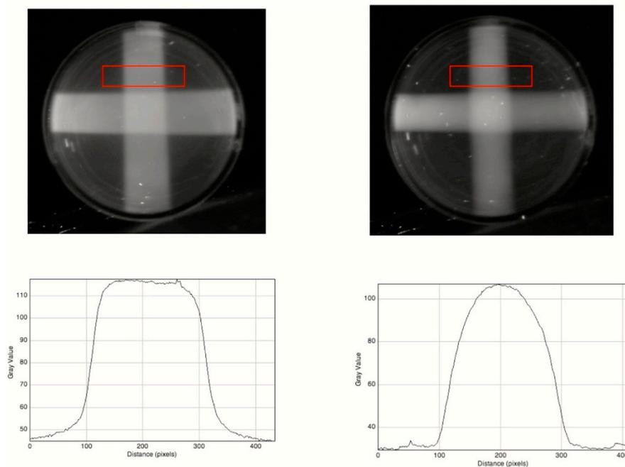
**Figure 11.** A 20 mm thick RFG gel irradiated with orthogonally-crossed X-ray beams. **Upper left:** a 10 × 10 mm square beam, **Upper right:** a 10 mm diameter round beam. **Lower:** pixel profiles across the beams as shown by the red rectangles. Pixel resolution 0.049 mm/pixel.
