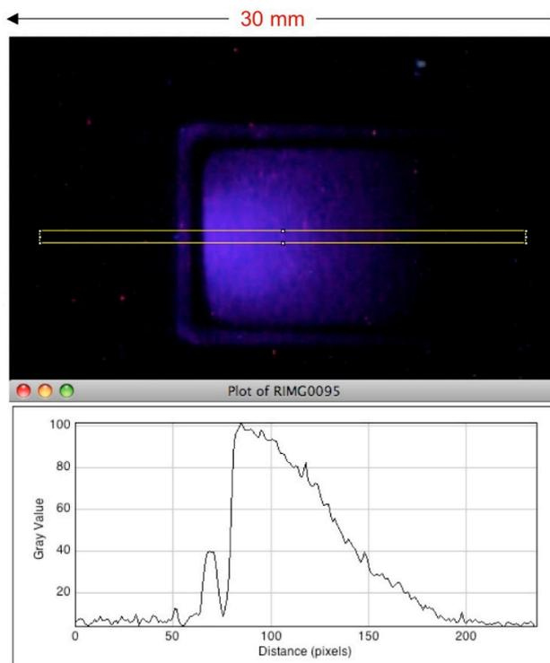
**Figure 6.** Upper: The depth-intensity image of the fluorescence of an RFG gel irradiated with a 3 mm diameter 3 MeV electron beam from a Van de Graaff accelerator. The yellow rectangle defines the limits of the plot-profile z-axis scan of the intensity shown in the lower part of the Figure. The pixel resolution was 0.11 mm per pixel. Taken from reference [26] Figure 9.
