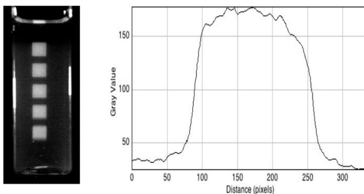
**Figure 7.** Left: A 20 mm square cell containing a 60 mm length of an RFG gel irradiated five times with a 5 mm square X-ray beam (dose 10 Gy) with the beams vertically displaced by 10 mm between irradiations. Right: A pixel profile scan across the central beam at 0.030 mm per pixel.
