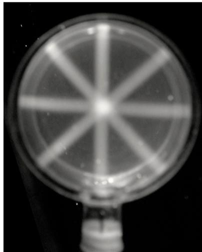
**Figure 10.** The fluorescence of a 6 mm thick RFG gel in a 50 mm diameter cylindrical quartz cell after irradiation with a 2.5 mm collimated, 250 kVp X-ray beam at 0, 45, 90, and 135 degrees to the vertical.
