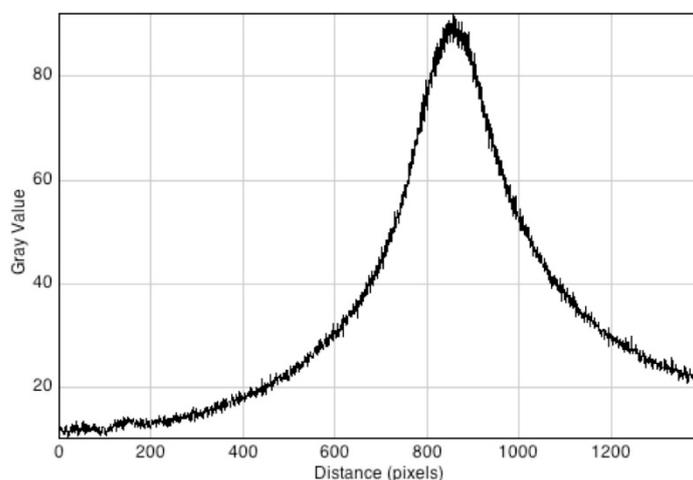
**Figure 16.** A pixel profile scan taken along the axis of the catheter, i.e., the centralvertical axis in Figure 15. The pixel resolution is  $0.035 \text{ mm/pixel}$  with a total scan length of approximately  $50 \text{ mm}$ .
