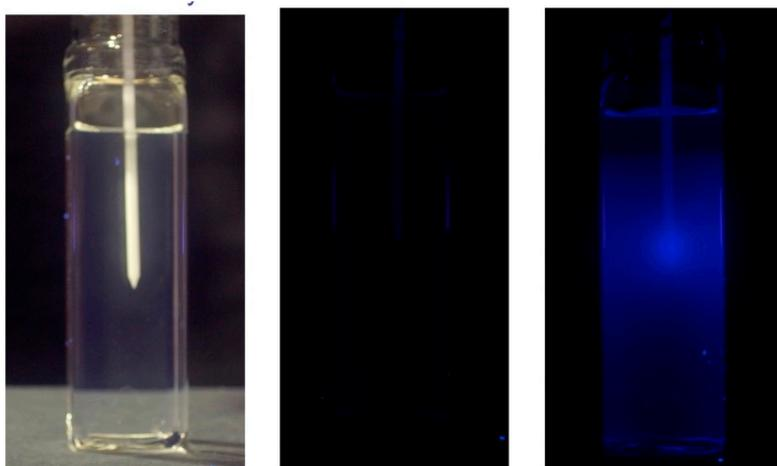
**Figure 15.** A  $20 \times 20 \text{ mm}^2$  square, 60 mm long RFG gel with a catheter inserted via a septum seal for insertion of a high dose rate seed of Iridium-192. **Left:** In room lighting prior to seed loading. **Middle:** In UV light prior to seed insertion. **Right:** In UV light 3 minutes after seed insertion.
