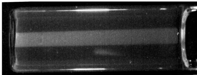
**Figure 8.** The image of a  $5 \times 5 \text{ mm}^2$  200 kVp X-ray beam propagating in a 60 mm length of RFG gel contained in a  $20 \times 20 \text{ mm}^2$  cell. Optical artifacts occur at the glass/air sides of the cell and at the gel meniscus.
