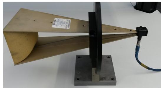
Figure 3.7: The TEM horn antenna
