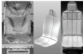
Fig. 2. Three stages in the seat development of the light weight seat: measuring the human contour (left), the CATIA 3d model (middle), the seat shell with inflatable cushions (right).
