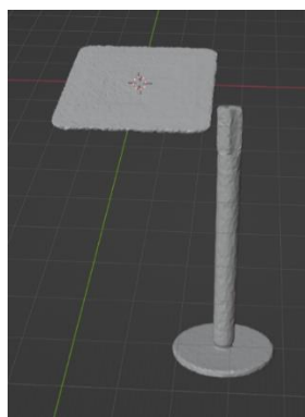
← Figure 22. Circular implant model. The 3D printed implant with attached ArUco marker was scanned with CBCT. The ArUco marker was manually aligned with Blender's x/y-plane.
