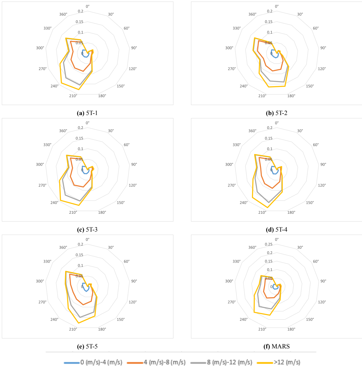
Figure 6.3: Wind rose diagram for the 5T wind farm
