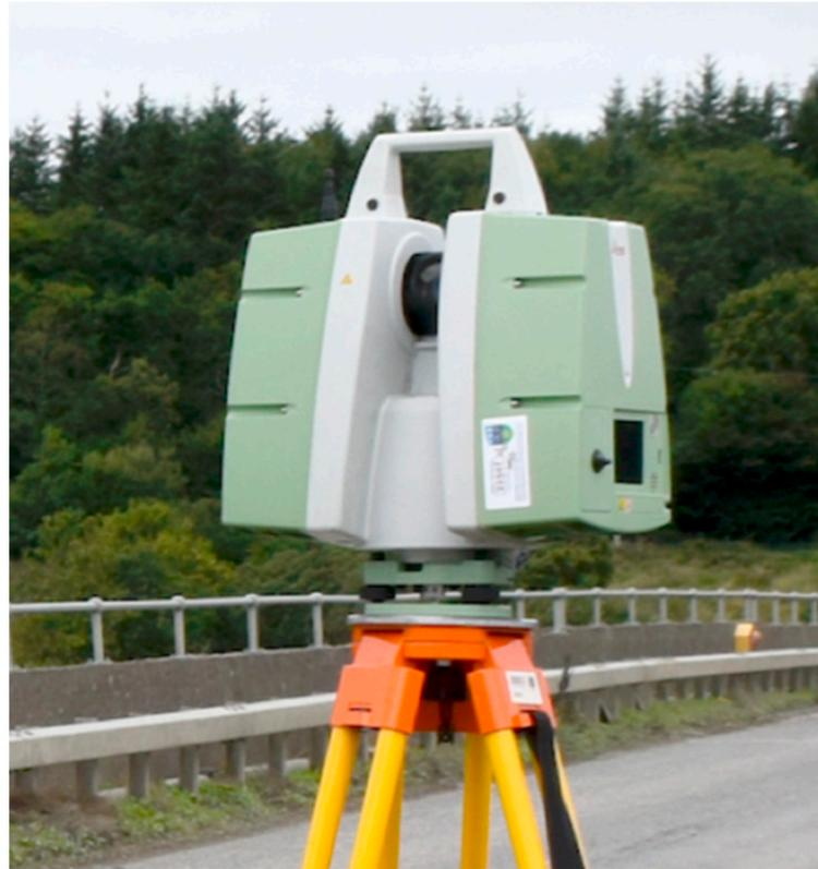
**Figure 12.** P20 laser scanner.
