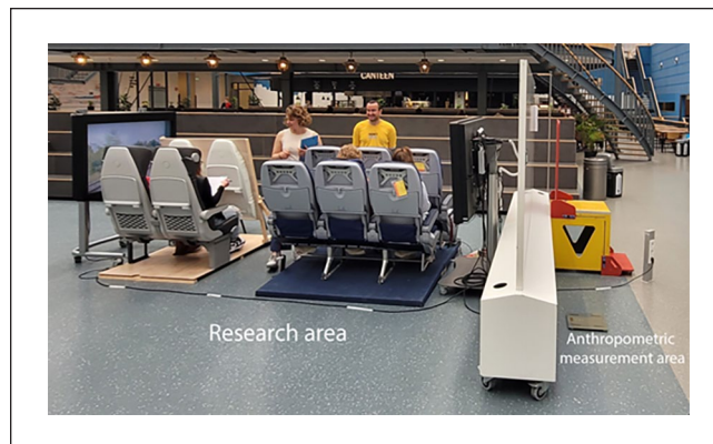
Fig. 1. Overview of the test set-up with 2x2 participants seated (2 in the train seat (left) and 2 in the aircraft seat (right)).
