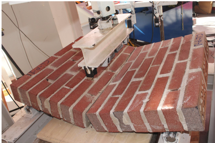
Figure 3.5: Out-of-plane bending tests conducted on perforated clay bricks (outer leaf).
