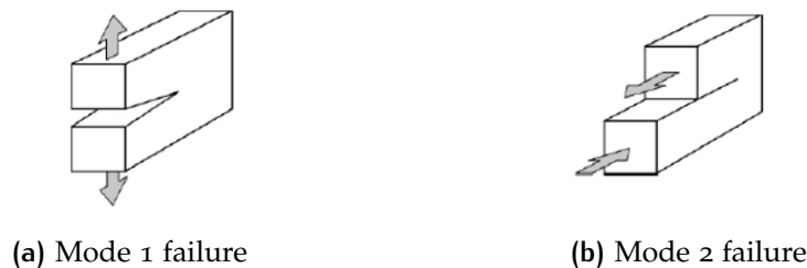
Figure 2.5: Modes of failure of tensile and shear behaviour respectively after Van der Pluijm (1992) [20]
