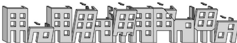
Figure 2.8: Examples of out-of-plane damage to masonry buildings
