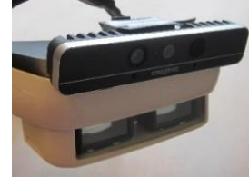
Fig. 3. Cinoptics AIRO II HMD for AR with the Intel® RealSense F200 mounted on top of it.
